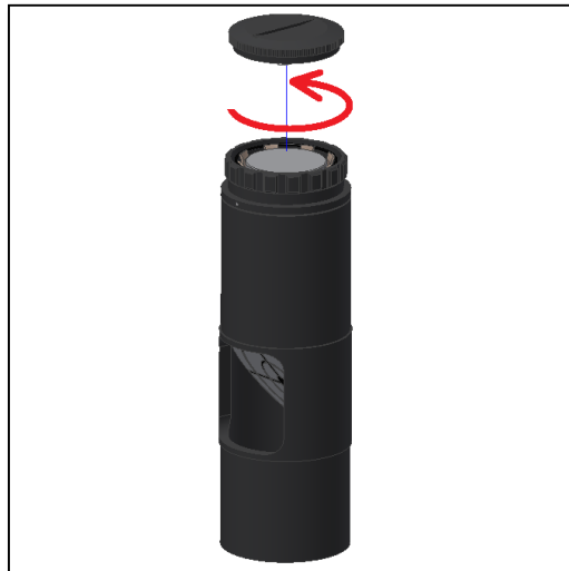
Figure 1. Remove cap to expose battery.
