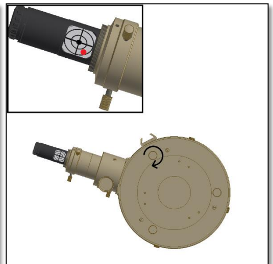
Figure 4. Rotate the laser viewer window so when adjusting the primary mirror the laser point can be seen.
